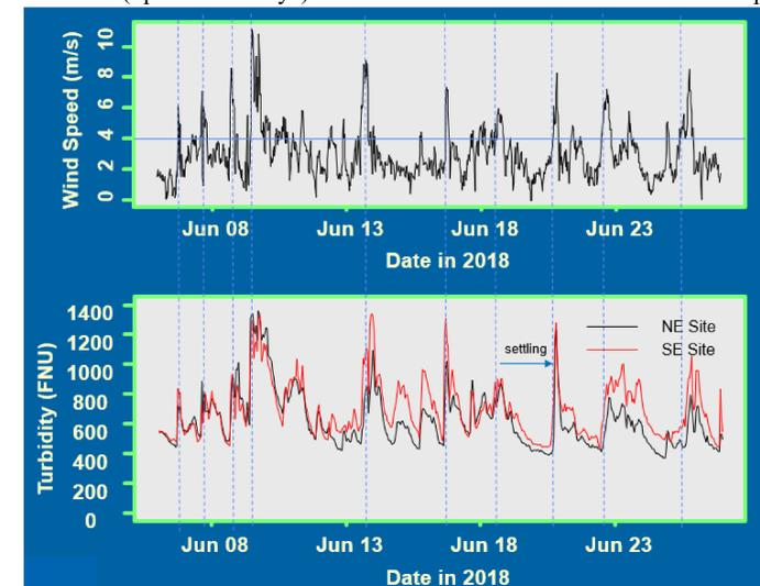
Figure 7. Continuous wind speed data and continuous turbidity data collected in Malheur Lake in 2018. Continuous turbidity data were collected at two sites within the lake (northeast [NE] and southeast [SE]). Vertical dashes align turbidity peaks with wind events.
