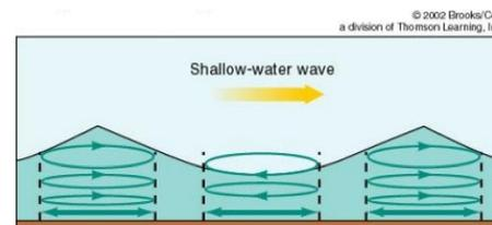
Figure 6. Shallow-water wave action. The back-and-forth movement associated with shallow waves creates shearing action at the lake bottom that lifts sediments into the water column.
