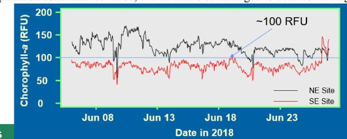
Figure 8. Continuous chlorophyll-*a* data (measured in relative fluorescence units) collected at two sites (northeast [NE] and southeast [SE]) in Malheur Lake in 2018.
